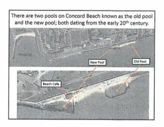
The old pool was originally a swimming pool made of wood; later concrete walls were added. In 1985 the present pool was built, using steel piling and concrete, inside the perimeter of the old wall. Later the pool was filled with sand to make it a paddling pool with a maximum depth of 18 inches.
