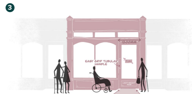
Accessibility - Shopfronts should cater for all abilities wherever possible. Strategies for achieving this include providing level access, a door width of at least 1200mm and a light-weight door with a push/pull sign and easy grip handle.
